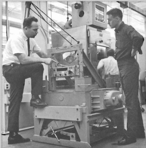
Environmental Testing subjects instruments to severe conditions. Jerry Chamberlain explains shaker table.
