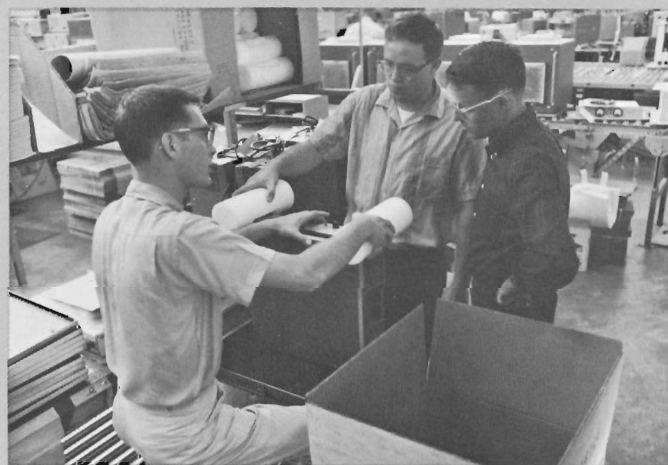
Don LaVoy (left) and Dave Bardin show how HP-designed post pack protects instruments against shock during shipment.
