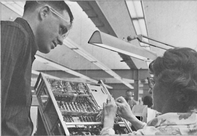
Lorna Nelson explains intricate wiring of 5245L counter. After few months' experience, women memorize entire wiring procedure.
